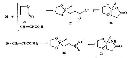
The formation of 24 and 26 is explained by the addition of 20 to the acrylic olefin bonds followed by hydrogentransfer, e.g. Thus, the adducts are reasonably deemed as the key intermediates, which react in the forms of zwitterions, 23 and 25. The reaction between two molecules of 23 is
