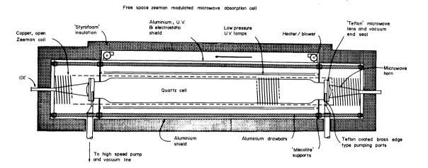
Fig. 5. Free space Zeeman-modulated quartz cell used for study of radicals.
