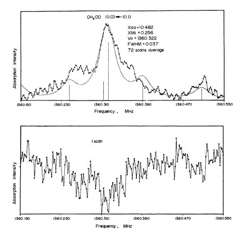
Fig. 4. Deuteromethanol line at 1.3603 GHz observed in L-band microwave spectrometer: (lower) single scan, (upper) computer averaged 72 scans and computer-filted multiplet superimposed.
