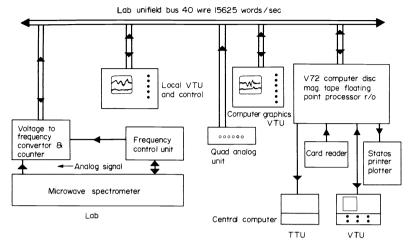
Fig. 3. Block diagram of spectrometer/computer combination used at Monash University.
