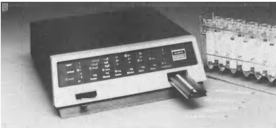
Fig. 8 Automated instrument for reflectance reading of reacted urine dip-and-read reagent strips.
