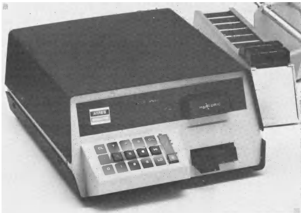
Fig. 7 Seralyzer, a reflectance colorimeter used with dry chemistry reagents to measure urea and other serum analytes
