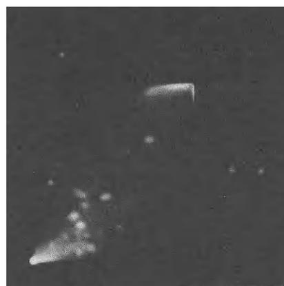
Fig. 6. Separation of an extract of peanut butter submitted to two-dimensional TLC (level of contamination ca. 5  $\mu\text{g}$  aflatoxin  $\text{B}_1/\text{kg}$ ;  $\text{B}_2$ ,  $\text{G}_1$  and  $\text{G}_2$  also present)
