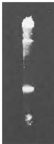
Fig. 4. Adsorption of aflatoxin B<sub>1</sub> on the Florisil<sup>®</sup> layer of a minicolumn according to Romer (ref. 12)
