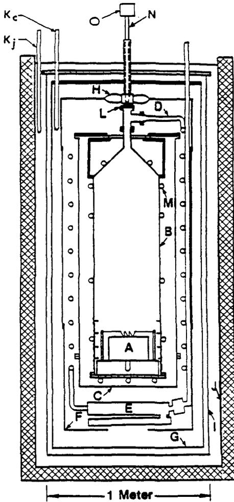
Fig. 1. Diagram of the multi-kilogram capacity flow calorimeter
