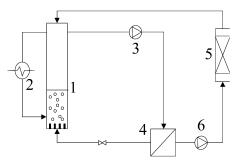
**Fig. 1** Schematic presentation of a reactor for the continuous enzymatic production and downstream processing of glucosides: (1) spray column reactor, (2) water bath (50 °C), (3) gear pump, (4) membrane module, (5) adsorption column, (6) plunger pump.
